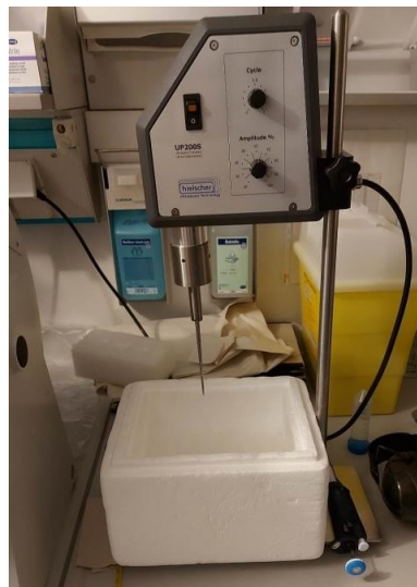
Figure 10. Working system used in sonication-assisted decellularization methods
