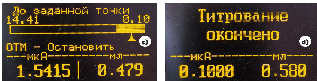
Figure 2. Data obtained at assay of a solution to be analyzed of Ferimax syrup by automatic amperometric method with two Pt indicator electrodes polarized up to 0,1 \mu\text{A} current intensity with \text{Na}_2\text{S}_2\text{O}_3 standardized solution without the addition of acetate buffer: a) at the beginning of titration; b) in the zone farthest from the equivalence point; c) in the zone near the equivalence point; d) the titrant volume at the equivalence point. ( V_0=50,0 ml; V_1=2,50 ml; m=0,8681 g; \rho=1,2404 g/ml; F=1,073 )
