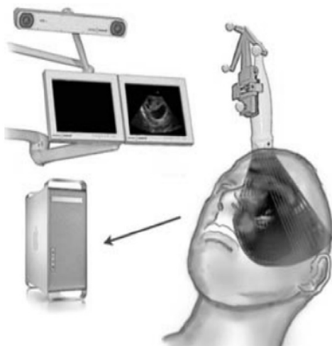
Fig. 3. 3D US image acquisition is done during the operation every time it is needed. The probe is moved over the region of interest, while each of the 100–200 images with the position data is tagged from the optical tracking camera and reconstructed into a regular 3D US volume. It takes about 30 seconds to create a new 3D US volume [1].
