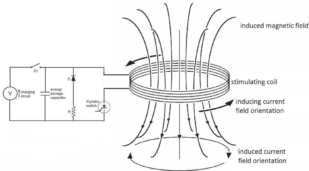
Fig. 1. The principle of the magnetic stimulator.
